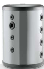
BTS TANK 100 or 150 litre separation buffer tank which reduces the on / off cycles of the compressor, reducing consumption and lengthening the life of the outdoor unit. The incorporated heat exchanger coil allows the separation of the primary circuit in the outdoor unit from the circuit from the house, being able to use glycolated water as heat-transferring fluid of the outdoor unit thus avoiding frosts, in the case of prolonged power cuts.
