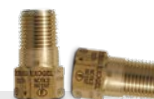
FROST PROTECTION VALVE Prevents the primary water circuit of the installation from freezing. In case of prolonged power cuts at extreme temperatures, it reduces the risk of the heat transfer fluid freezing by draining the outdoor unit circuit.
